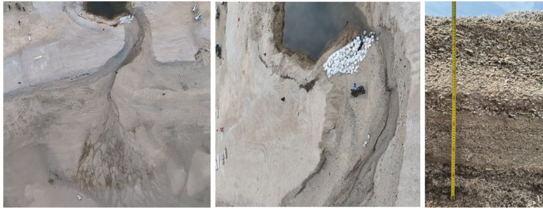
Figure 4. Formation of a Large Erosion Trench in the Dammed Lake at Shiluokou Due to Storm Surge (Photographed on 2024.9.16)
