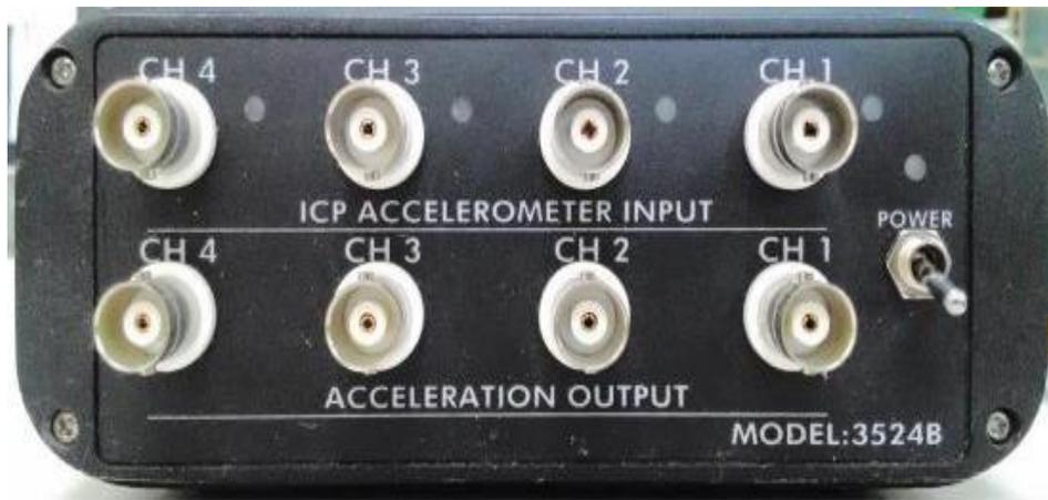
Figure 3. Left side view of the house Integrator
