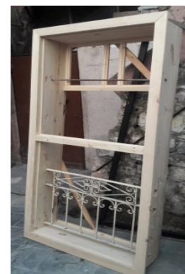
Figure 33. Fabrication of patterns of window casement, sash, muntins, and Iron bars (Hammoud J., 2021)
