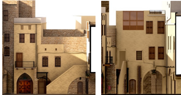
Figure 22. Design of the façades in Furn el Saha square. Timber doors, windows and musharbiyyeh are restored and walls address both aesthetic and functional concerns (Hammoud J., 2022)
