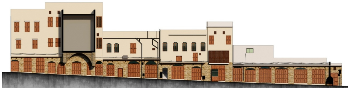
Figure 19. Design of the façade in Musallabiyyeh old market street involving a balanced blend of sensitivity and innovation. The design effectively differentiates the concrete parapet that is white in colour. The upper part of the façade is lime plastered while the market level is kept stone due to the local residents' request. The sanitary pipes are shown in black colour adding visual interest through contrast (Hammoud J., 2023).
