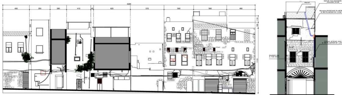
Figure 12. Architectural drawings recording the existing situation of the facades in Musallabiyeh old market street (Hammoud J., 2022).
