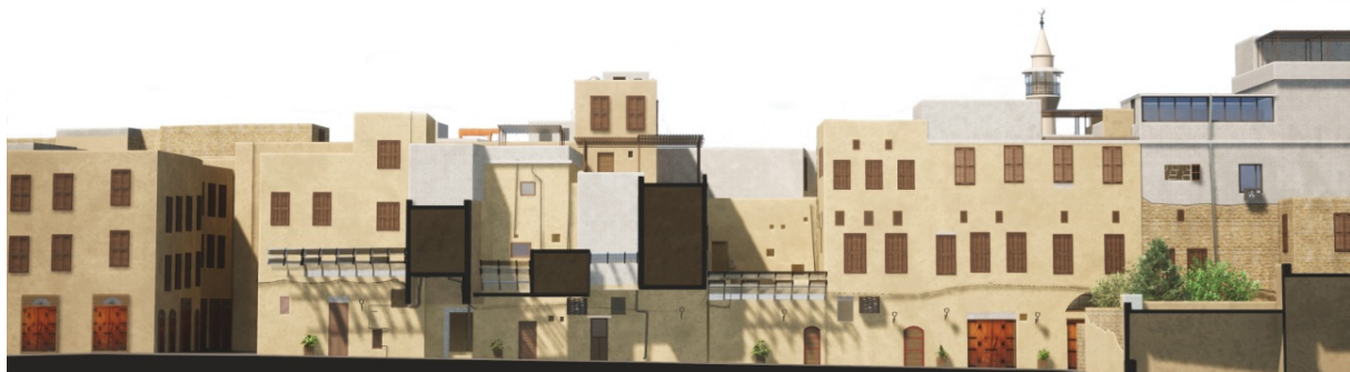
Figure 20. Design of the façade in Kaniset el Amercani street showing its overall historic character. Timber doors and windows are restored, walls are lime plastered and the existing additions introduce distinct visual elements to the concrete portions coloured in white (Hammoud J., 2022).
