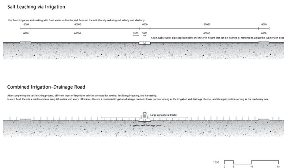
Figure 5. Schematic of the “irrigation-drainage integrated road” system
