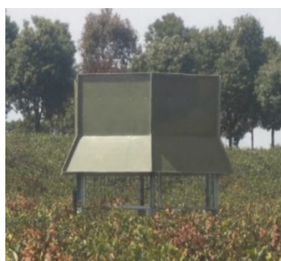
Figure 4. Suction-exhaust wind machine
